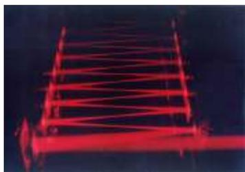
**Fig T.1.6b** Simulated beam path and multiple focal volumes produced by He-Ne laser.
