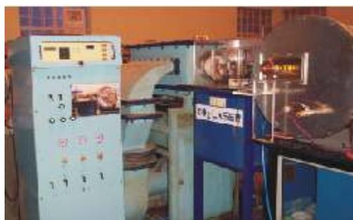
**Fig T.1.7** TEA CO<sub>2</sub> laser and large irradiation cell of 110 liter
