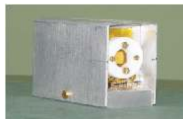
Fig L.4.2 Bolometer detector assembled in the metallic housing
