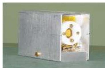
**Fig L.4.2** Bolometer detector assembled in the metallic housing
