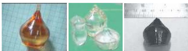
Fig. L.16.1 As grown undoped, Mg and Cr doped LN crystal boules
