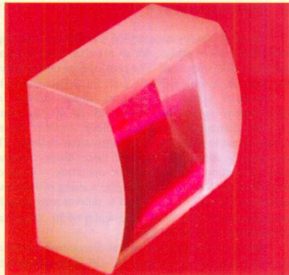
Fig. L.13.2 Plano convex lens of size 50x45x25mm with radius 50mm from BK7 glass.
