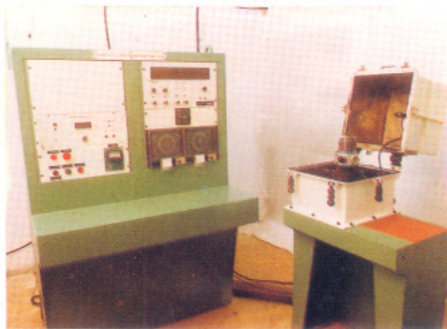
High-speed-assembly balancing machine for turbomolecular pump.
