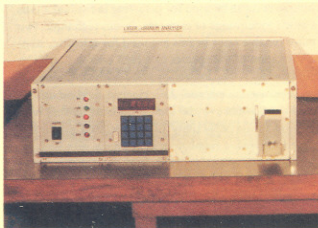
Fig. 4. Laser uranium analyzer developed at CAT. Top photograph shows the inner view of a unit. From left to right are the nitrogen laser system, power supply and the processing cards. The front panel has displays for nitrogen gas pressure, upper and lower limits set for the laser power and the measured uranium concentration. The bottom photograph shows the present prototype model assembled in a standard commercial rack of size 425 X 425 X 145 mm by optimising the various subsystems.
