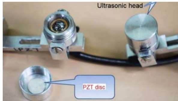
Fig.B.(10): (Left) In-house developed module for low intensity ultrasound generation and (right) magnified view of ultrasonic heads, carrying piezo-electric disc
