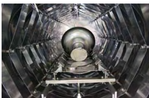
Fig.A.10 : Single-cell cavity loaded in furnace.
