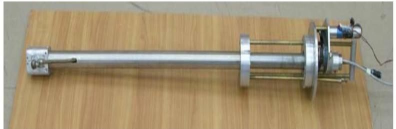
*Fig. 47: laser cutting tool for liner tube and end-fitting.*
