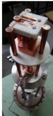
*Fig 56(b): The chip-mount assembly.*
