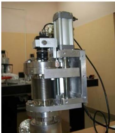
*Fig. 5: Photographs of BPM and bellow assembly during lab test.*
