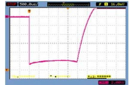
Fig. 33: Typical saturated bolometer trace during lasing.
