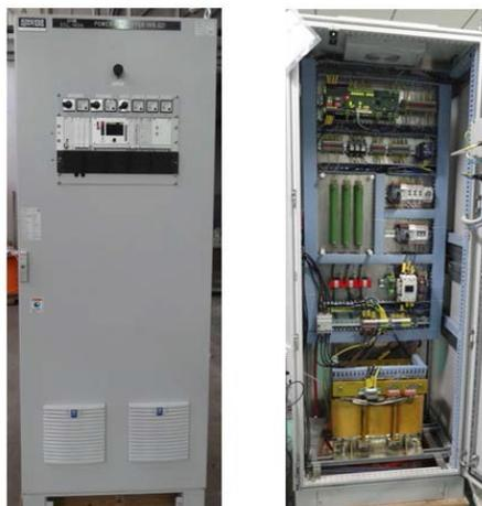
Fig. 70: A photograph showing the power converter for electromagnet developed for FAIR.
