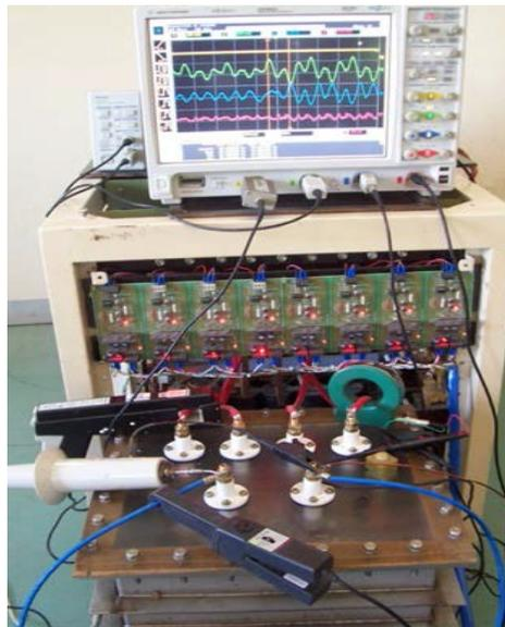
*Fig. 27: High voltage capacitor charging power supply during testing.*
