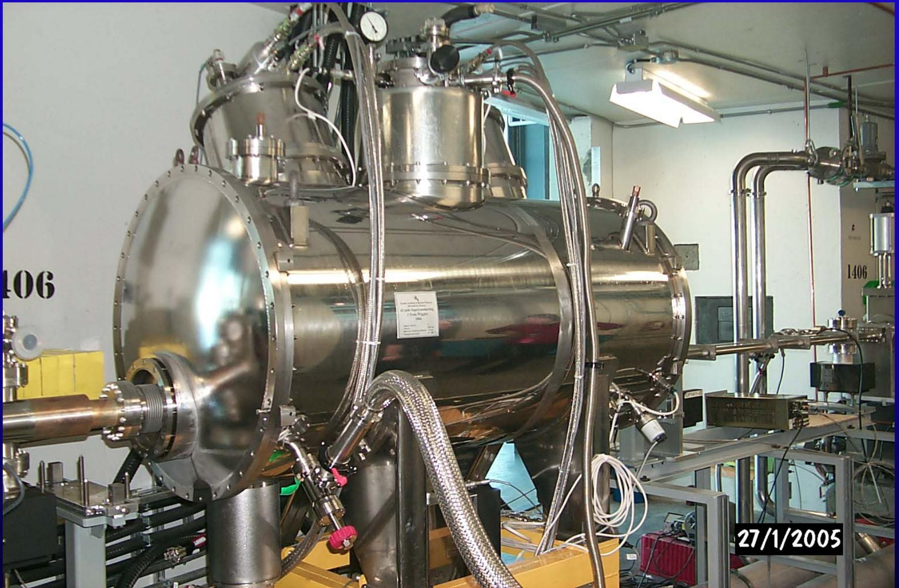
**Superconductive 2.2 T 63-pole wiggler
