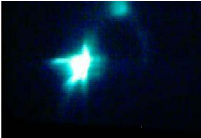
Synchrotron Light at 2mA Beam as seen by CCD on Feb 17, 2006
