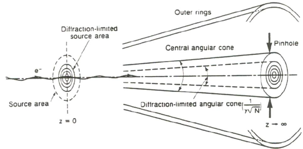
Illustration of the diffraction limited angular emission from an electron traversing an undulator structure. In practice the finite emittance of the beam increases the diffraction limited source area and divergence.
