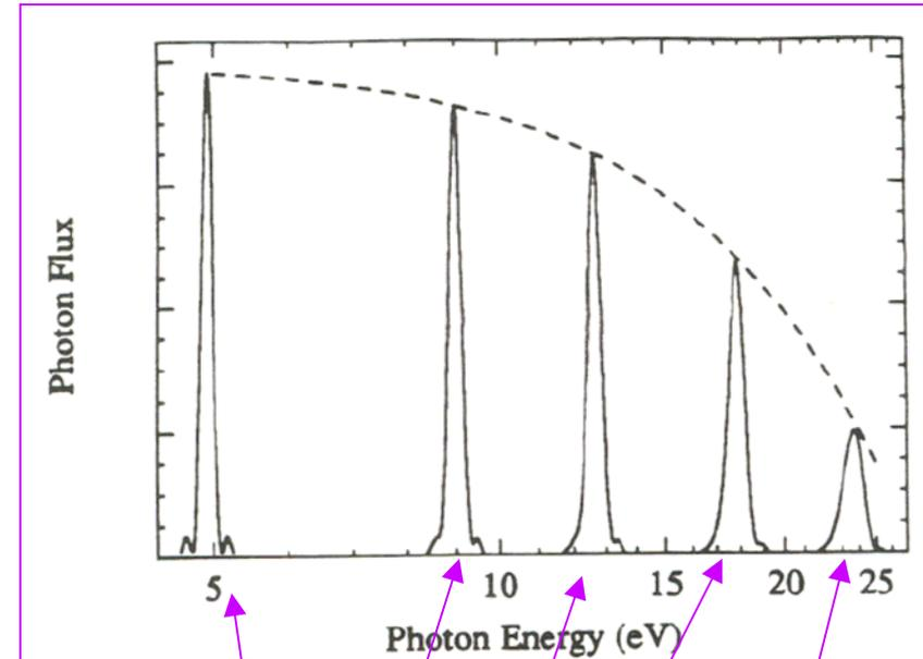
**First harmonic peaks as a function of  $K$  for, left to right:  $K = 3.0, 2.0, 1.5, 1.0$  and  $0.5$ . Undulator for this example has a period of 87 mm and 29 periods.  $V=0.5$  GeV. Envelope of peaks gives tuning curve of the (variable gap) undulator.**
