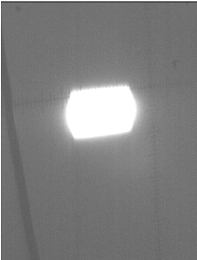
**SR as seen on the Be window of the EDXRD beam line (BL11).
