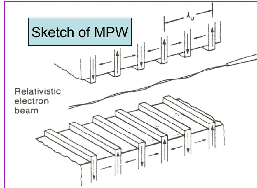
Schematic of a multipole wiggler/undulator using a hybrid construction of permanent magnets and steel poles.
