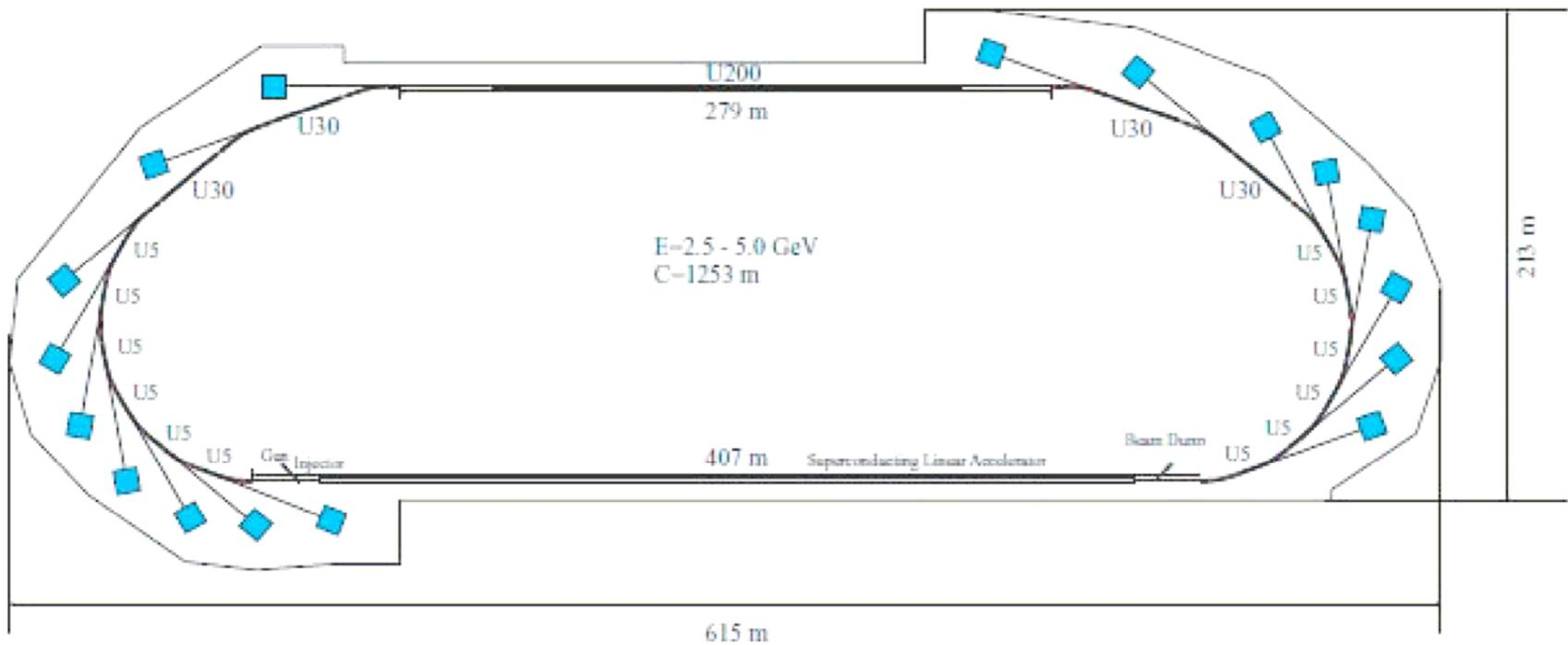
Figure 2. The 2.5 to 5 GeV, 100 mA Energy Recovery Linac under consideration at KEK is designed to provide next generation capability for users of the Photon Factory. Seventeen x-ray beamlines from 5 and 30 meter long undulators are shown in this schematic layout.
