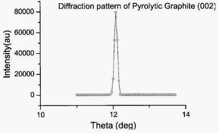
**First x-ray diffraction record with SR from Indus-2 using XRD BL12 on Sept 28, 2006; Indus-2 beam energy was 2 GeV & current ~4 mA. DCM was aligned to get monochromatic SR out but calibration was still on. Collecting and focusing mirrors were not yet in place.**
