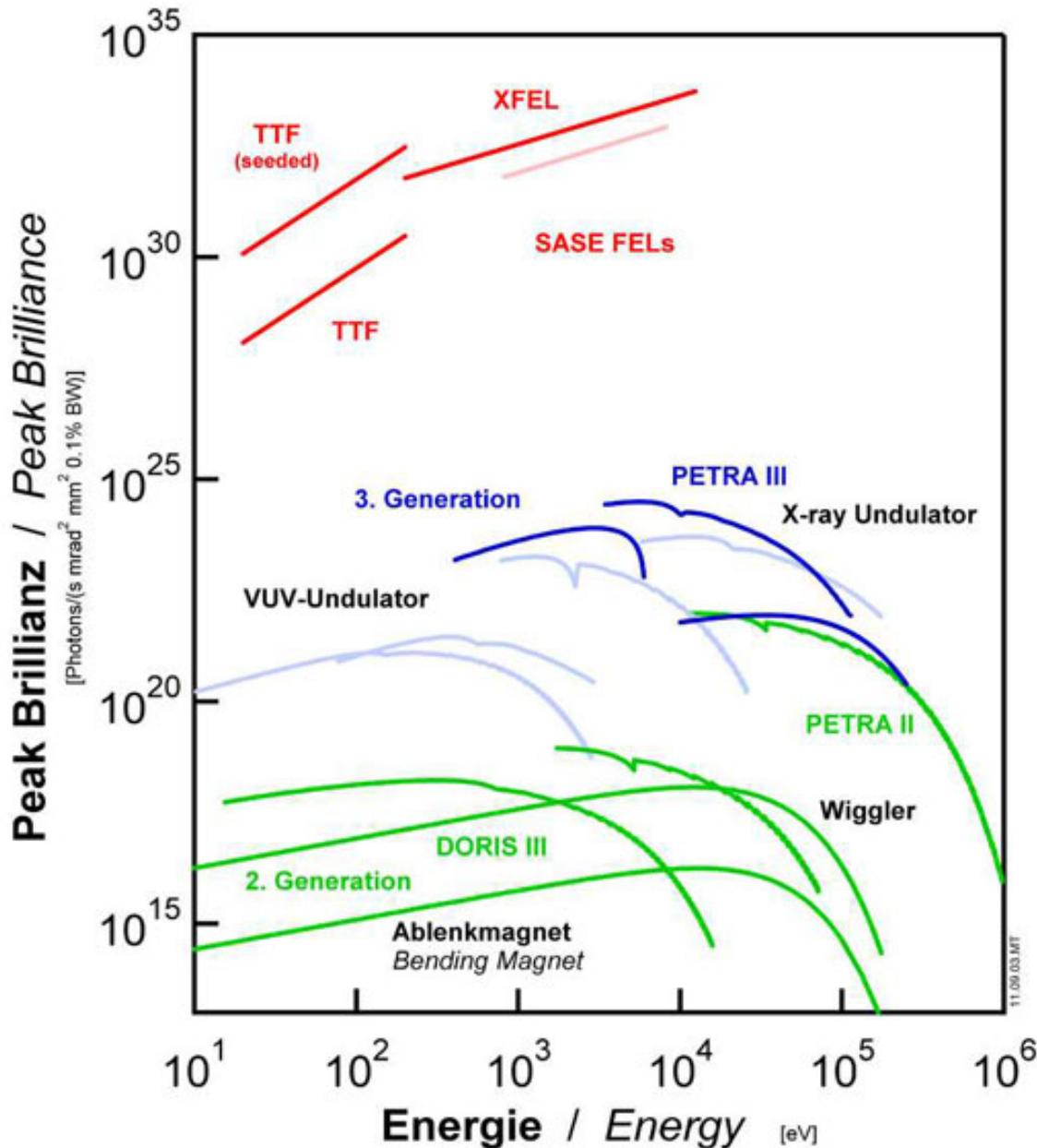
This comparison of peak brightness of synchrotron radiation sources with free-electron lasers (FELs, red lines) shows the great leap in brightness offered by the FELs. (Source: DESY Hamburg)
