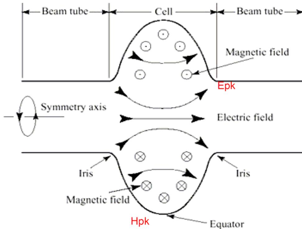
Note that the EM field will accelerate & impart energy to the electrons if they are in phase with the electric field. But if electrons see the electric field  $180^\circ$  out of phase, then EM field will decelerate them. Then the EM field will gain energy from the electrons. This is the “energy recovery” idea used in ERLs.
