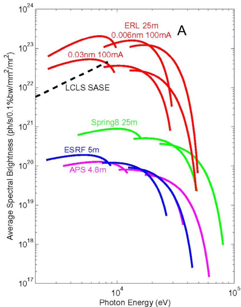
Figure A shows the average spectral brightness vs. photon energy for a 25 m long ERL undulator<sup>16</sup>. As can be seen in the top curves belonging to the ERL (red), the average spectral brightness will be several orders of magnitude higher than existing storage ring sources and even higher than the average (but not peak) brightness of the LCLS.
