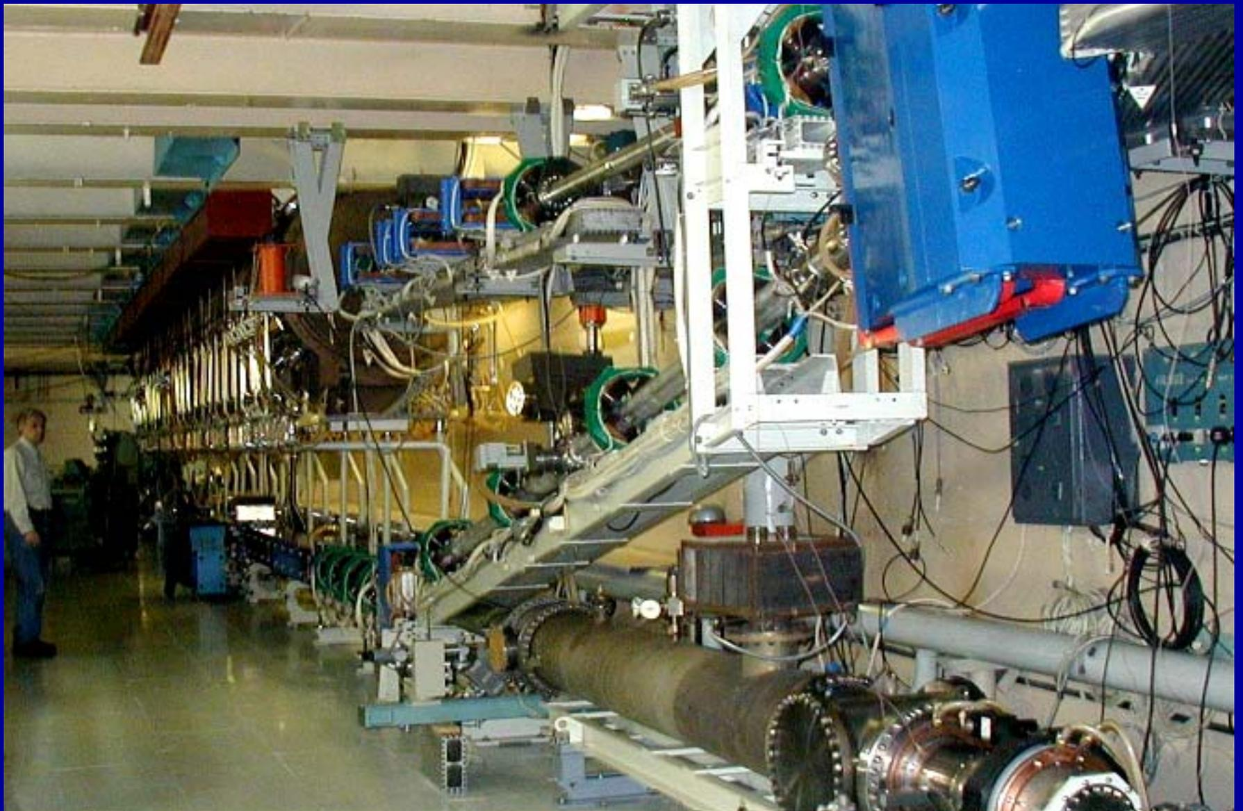
On April 4, 2003, first lasing was obtained at a 1st stage FEL. At present, this FEL is the most powerful (400 W) generator of the terahertz radiation with tunable wavelength (120-235  $\mu\text{m}$ ,  $\delta\lambda/\lambda=3\cdot 10^{-3}$ ).
