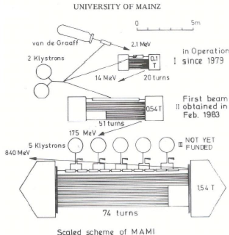
Figure 5.5 Schematic layout of the University of Mainz three-stage cascaded race-track microtron, MAMI (Herminghaus *et al.*, 1983; © 1983 IEEE)
