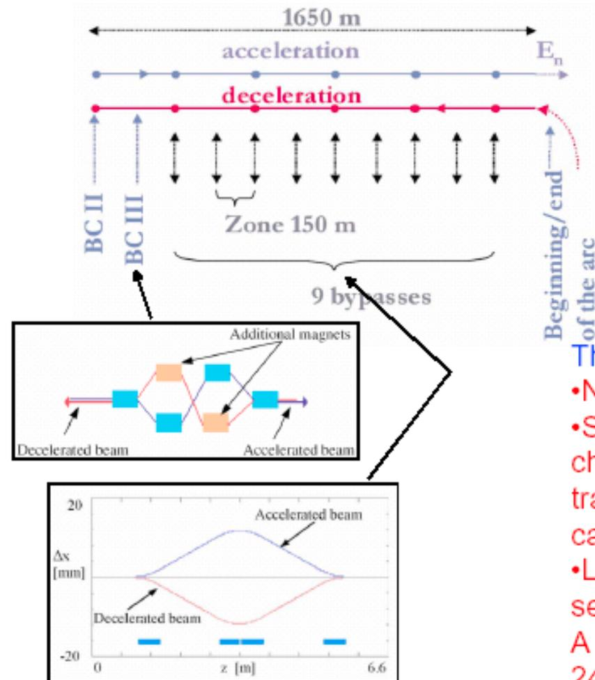
At a 1 MHz rep rate there are 6 bunches in the ERL at a given time, thus 12 collision locations separated by 150 meters.
