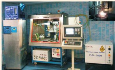
LAM system using Direct Energy Deposition
