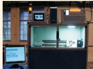
LAM system using Powder Bed Fusion
