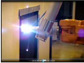
Paint stripping using CO2 laser
