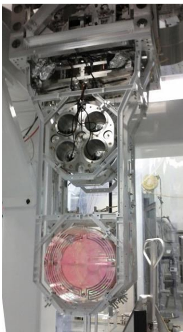
Fig. T.2.11: A photograph of one of the quad-suspensions used in aLIGO taken during assembly. (Credit: Caltech/MIT/LIGO Laboratory)
