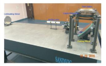
Fig. L.5.2: Photograph of the Liquid reference Fizeau interferometer
