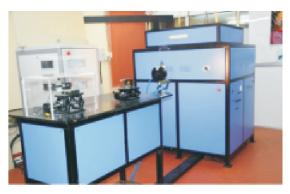
Fig. L.4.4: Upgraded 2 kW RF-FAF  $CO_2$  laser We operated the laser with a plano-concave stable resonator to obtain 1.1 kW at 10 kW RF input. The upgraded laser system with 20 kW all solid state RF source is shown in Fig. L.2.4.
