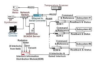
Fig. A.5.1: Architecture of new Control system of Microtron
