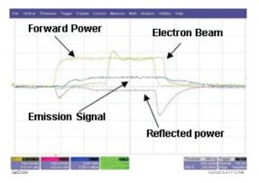
Fig. A.5.3: Various parameter waveforms on DSO
