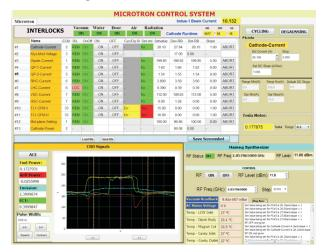
Fig. A.5.2: GUI for new Control system designed in WINCCOASCADA
