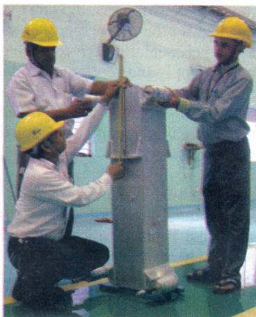
Fig.A.5.1: Aluminium Plate Fin Heat Exchanger developed for Cryogenics Application
