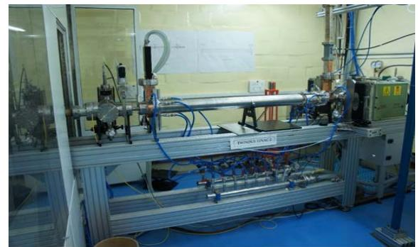
*Fig. 29: Second linac tested at beam power of 1 kW.*
