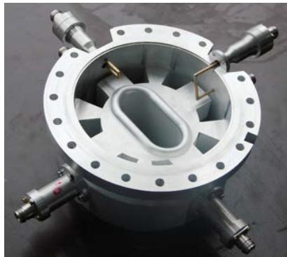
*Fig.11: Half cell of kicker RF cavity.*
