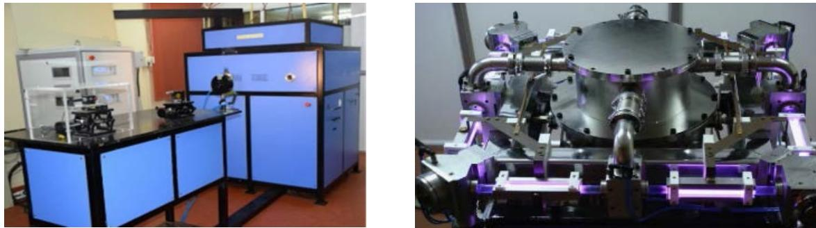
*Fig. 44: 2 kW RF-FAF CO<sub>2</sub> laser (left) and RF discharge in four sections of the laser (right).*
