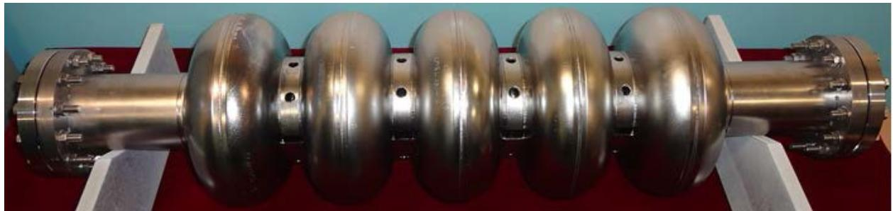
*Fig : 24-cell laser welded superconducting radio frequency cavity.*
