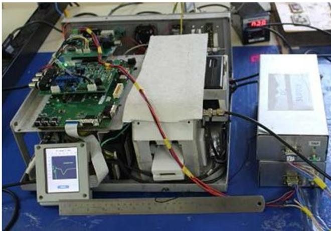
*Fig. 25: Oxygen detection on detector's screen with RRCAT HV pulse and HV DC supplies.*
