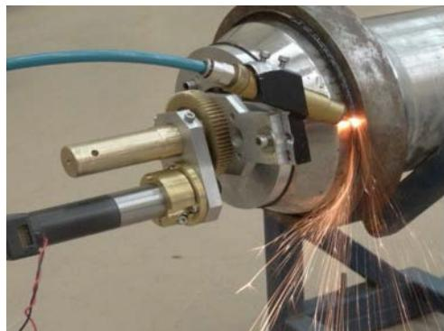
*Fig. 46: Mock-trial for laser cutting of bellow lip after removal of outboard end-fitting.*
